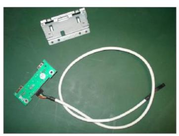
**10.4** Press the bottom hook on PCB holder, remove **PCB assembly**; Press two side hooks on PCB holder, remove **POWER SWTICH PCB**
